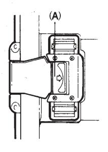
To remove the back cover opening lever (26), slide the lever's lock (A) in the arrow direction. Open the back cover by raising the lever with your finger.
