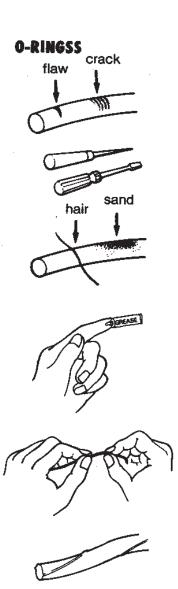
The MOTOR MARINE IIEX maintains its waterproofness by use of O-rings. In order to make the most of the O-rings, take the following precautions. Improper handling may cause water to get into the unit.
